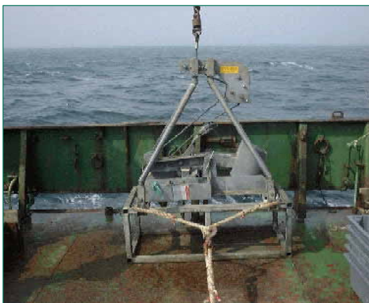
Figure 2 Hamon grab primed and ready for deployment. Note the winch controlled lateral supporting rope for increased stability and therefore safety during deployment and recovery. It is unhooked before the descent of the sampler
