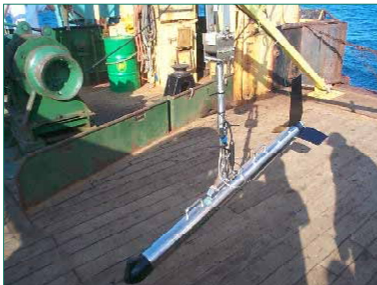
Figure 28 Datasonics™ SIS 1500 Chirp sidescan sonar fish. This device acts as a stable platform for the transducers, and is towed behind the vessel during the survey
