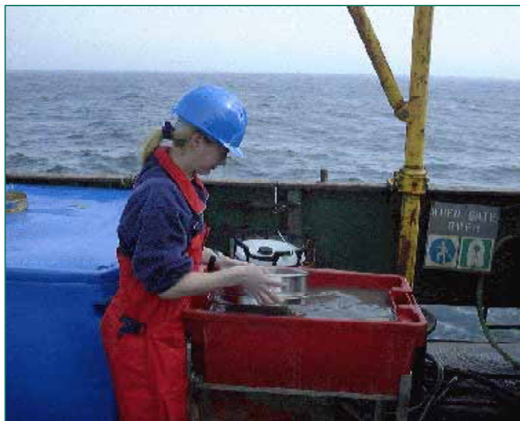
Figure 20 ‘Puddling’ - the removal of accumulations of fine sediment through gentle vertical motion of the sieve. Note that the seawater-filled container is placed at waist height for ease of processing
