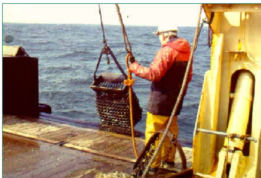
Figure 15 A Rock dredge. Note the heavy-duty rectangular metal rim and the collection bag consisting of interlaced metal rings
