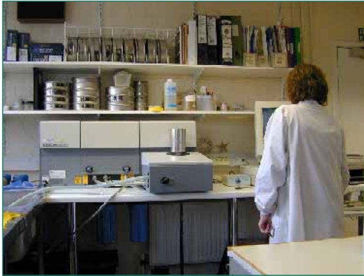
Figure 35 Coulter™ LS 130 laser sizer. This equipment uses laser diffraction technology to measure particle diameters. It is most frequently used to measure the finer component ( <500\ \mu\text{m}/<63\ \mu\text{m} ) of a sediment sample
