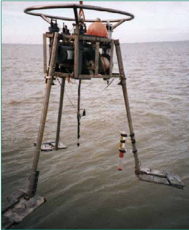
Figure 31 CEFAS Minipod. The Minipod consists of a hard-disc based burst logger, capable of recording the current velocities (from a Nortek Vector® Acoustic Doppler Velocimeter), pressure (using a DigiQuartz® sensor), suspended sediment sensors (acoustic for sands and optical for finer material) and seabed position. Passive and timed sediment traps (Booner tubes) are also evident on two legs
