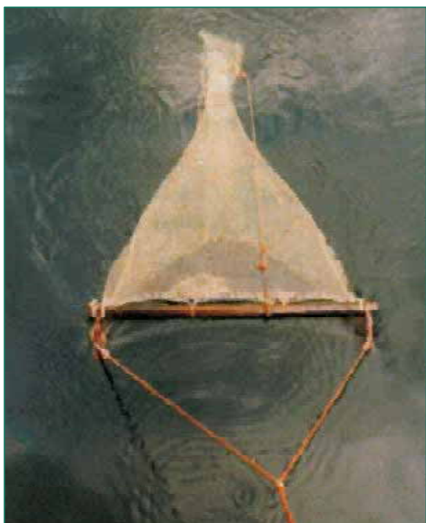
Figure 11 A standard Lowestoft 2-m wooden beam trawl (Riley et al. , 1986) at the water surface prior to deployment. Note the wooden 2 m beam and the pair of towing bridles attached to the trawl shoes
