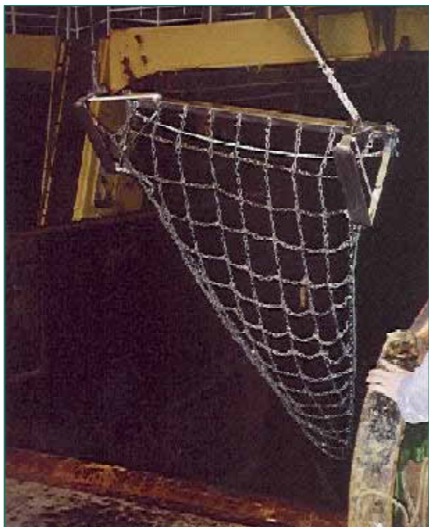
Figure 10 A heavy-duty 2-m beam trawl with chain mat being recovered over the stern of the research vessel. Note the metal beam between the two trawl shoes and the chain mat attached to the underside of the beam
