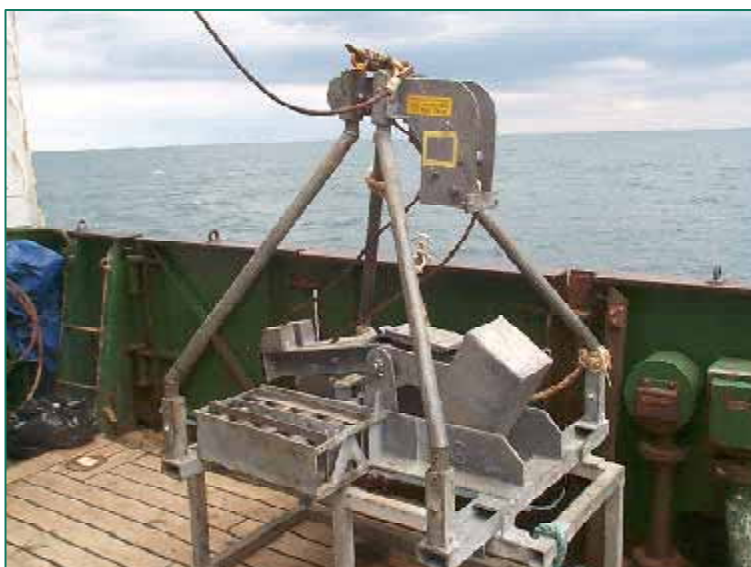
Figure 5 A 0.1 m 2 Hamon grab supported on an open frame to facilitate retrieval of the sample into a moveable container following controlled release from the bucket. Note the nearside rack supporting lead weights to increase sampler efficiency (a comparable rack on the other side of the sampler is hidden from view in this photograph)
